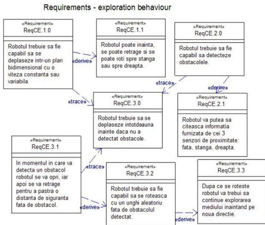
Fig. 2. Requirements diagram - exploration behaviour
