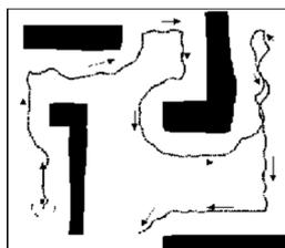
Fig. 6. Fuzzy behaviours in navigation – wall following behaviour
