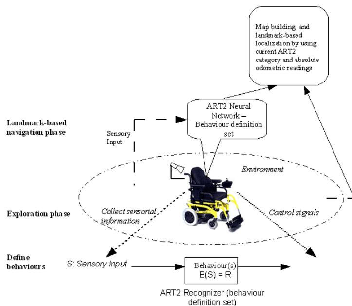
Fig. 2. Behaviour based navigation by using schemas theory
