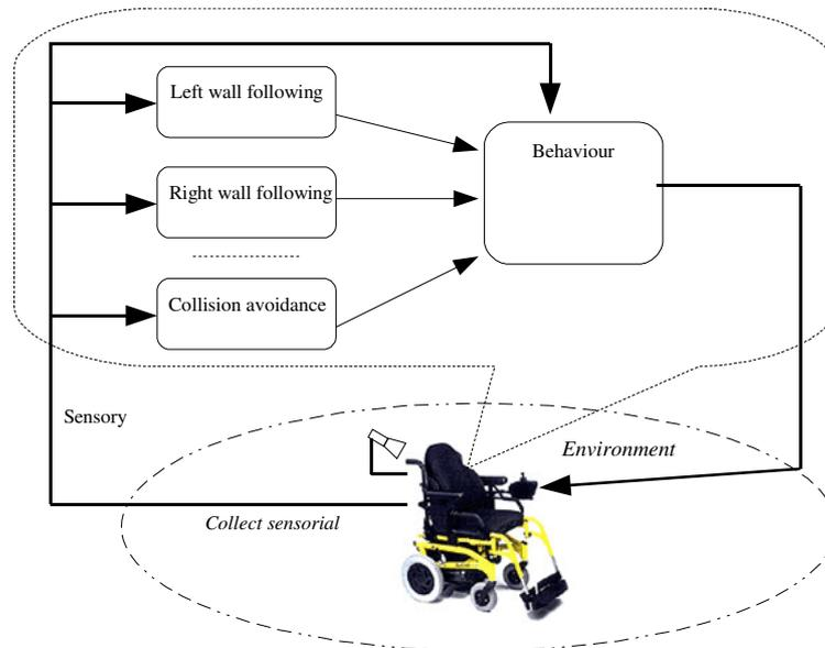
Fig. 5. Fuzzy multi-behaviour based controller for autonomous navigation
