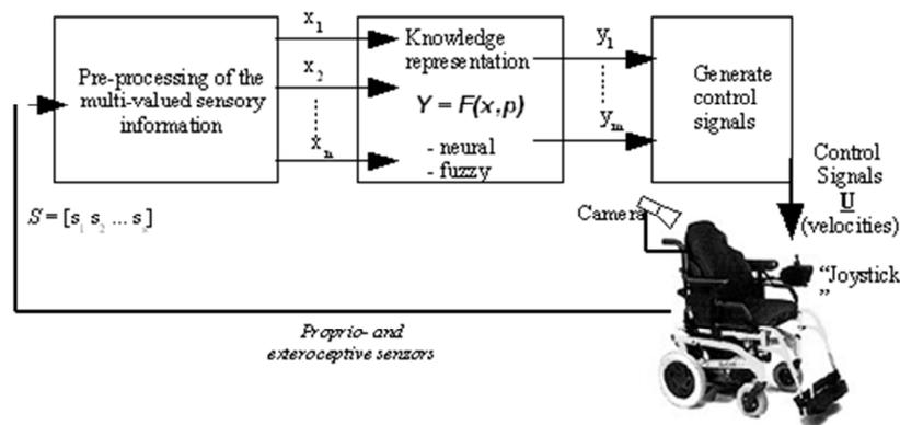
Fig. 1. Intelligent Transport System (ITT) for Accessibility and Mobility
