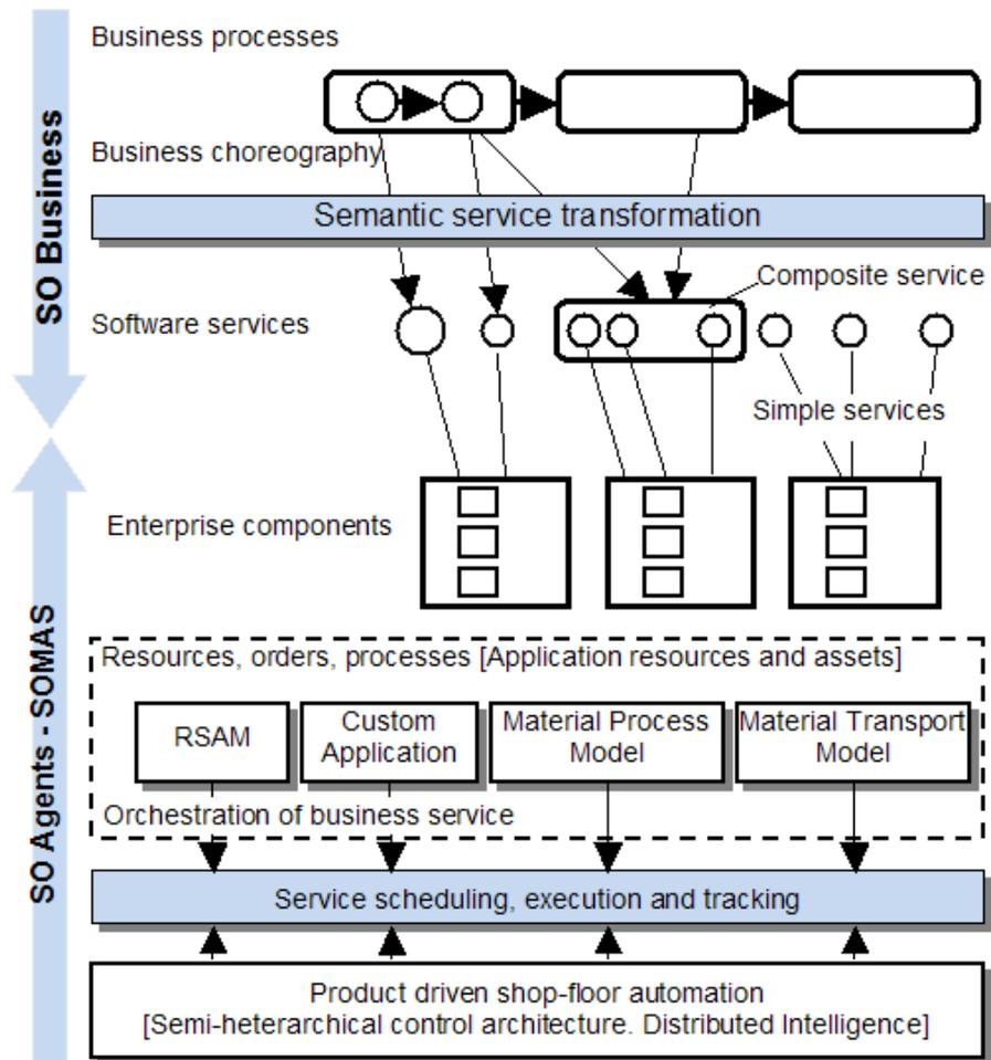
Fig. 8. The Service Oriented Enterprise Architecture for manufacturing
